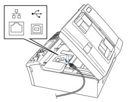
12 Carefully route the USB cable through the trench and out the back of the machine as shown below and connect the cable to your computer.
